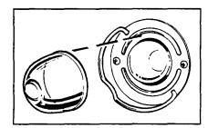
The oven lamp (bulb) is covered with a removable glass cover which is held in place with a bail-shaped wire. Remove oven door, if desired, to reach cover easily.
